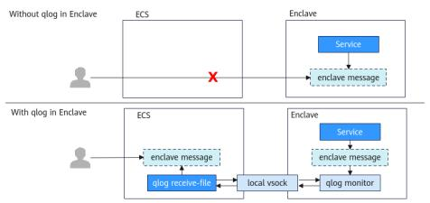
Figure 19-2 Seamless migration of a network service to QingTian Enclave
